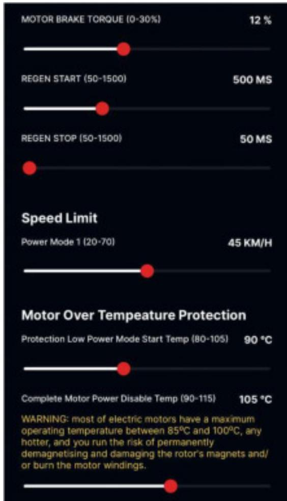
**Motor brake torque** – This is an adjustment for the strength of the regen braking. Below 5% will hardly be noticeable and up over 25% will be rather significant. Have a play to see what suits your riding style
